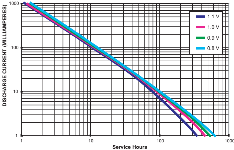
TYPICAL CONSTANT CURRENT DISCHARGE CHARACTERISTICS AT 21°C (70°F)
